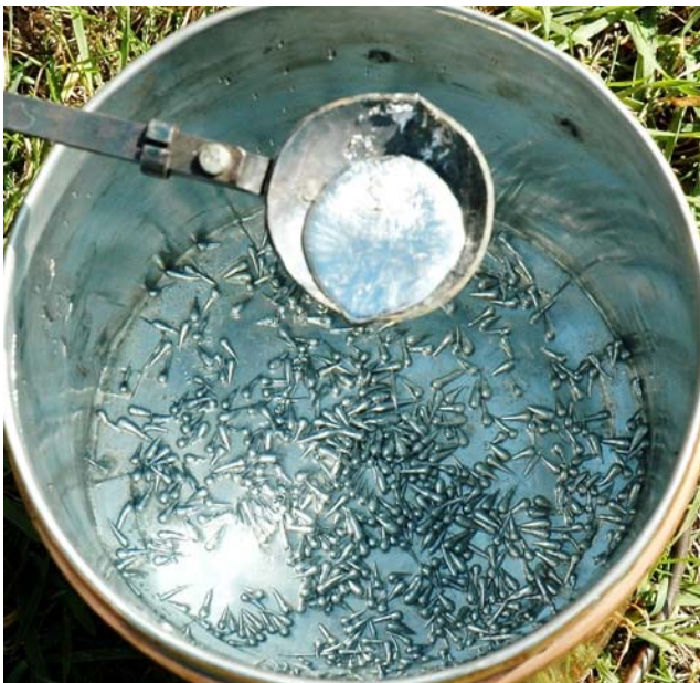
If the hypothesis is correct, making drip shot was a wilderness process born of necessity, requiring a few lead balls, a ladle, a campfire and a kettle of water.
