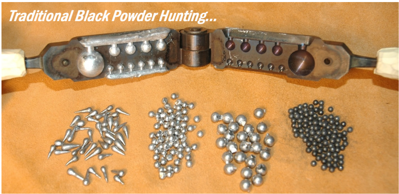
A 1790-era traditional hunter has a number of shot choices that include (left to right): homemade drip shot, "duck" and "swan" shot cast in the reproduction mold pictured, and #4 drop shot that replaced Rupert shot after 1782.
