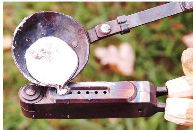
Rediscovering the old ways, like casting shot in a gang mold, requires careful observation, patience and a willingness to experiment until a proper technique can be mastered.
